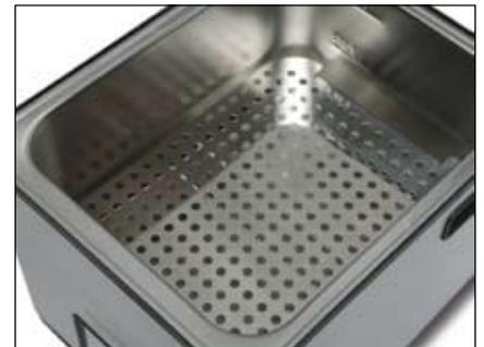
Bottom grill generates thermal convection currents for even temperature distribution.
